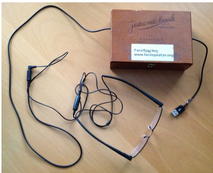
Figure 5: The FaceSpeaker camera box. On one side there is a single USB cable which is connected to the laptop. The camera glasses are connected to a cable coming out at the other side.
