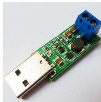
Figure 7: The 5W USB DC-DC 5V to 9V Step Up Boost Module. This voltage booster can be plugged into a standard USB port and outputs 9 volts of power from 2 terminals into which wires can be screwed.
