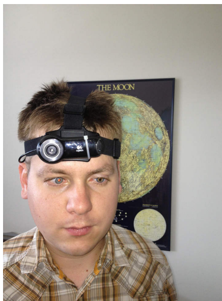
Figure 13: The FaceSpeaker author wearing a Logitech Pro9000 webcam mounted onto a headband
