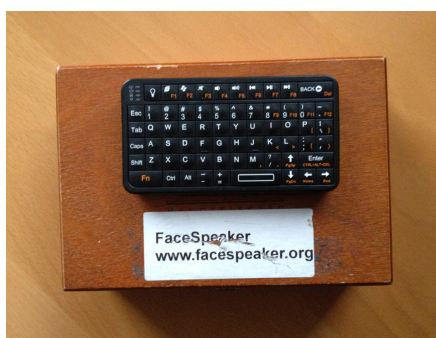
Figure 8: Riitek mini bluetooth keyboard used to control the FaceSpeaker prototype.
